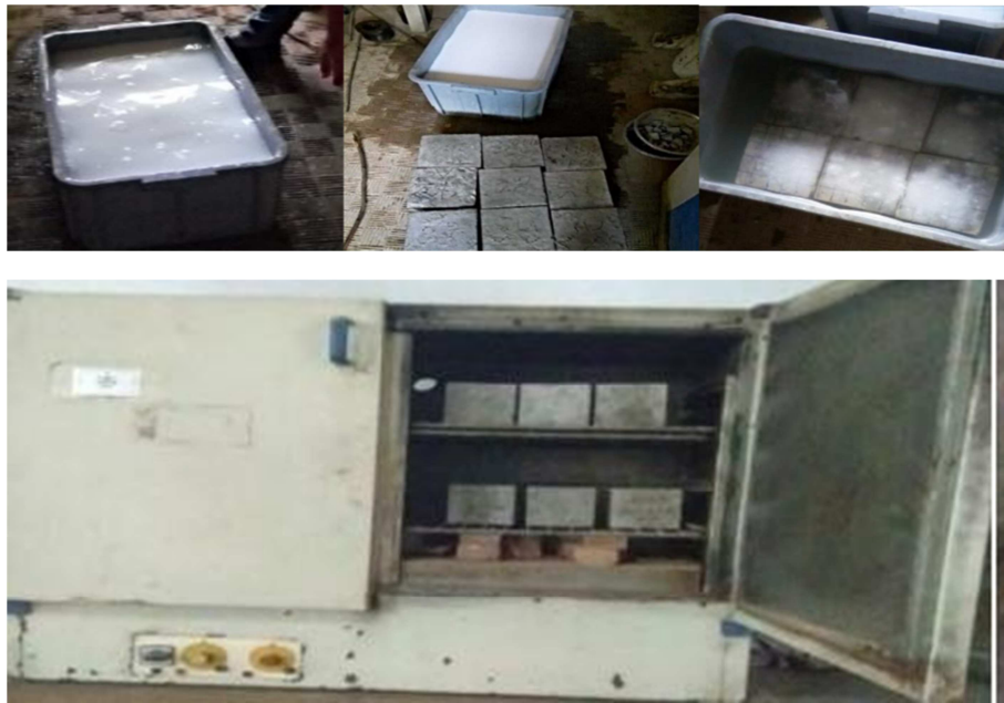
Figure 5. Solution of ammonium nitrate and magnesium sulfate and concrete specimens.
