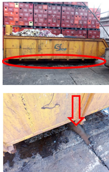
Figure 6. Casting leachate under the garbage bins.
