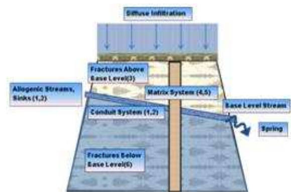
Figure 3.. Aggtelek aquifer conceptual model.
