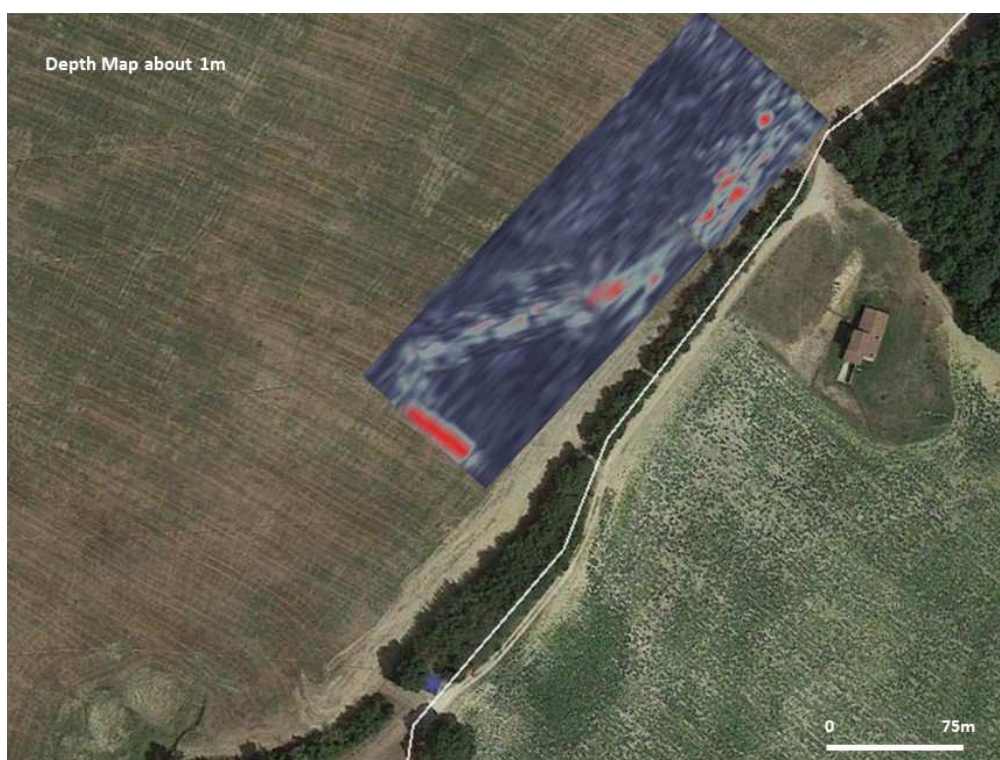
Figure 10. In this figure, it is possible to notice the elongated strong GPR anomalies in Area 3 at a depth of approximately 1.5 m. Due to their geometry, it is possible they are linked to ancient manmade structures.
