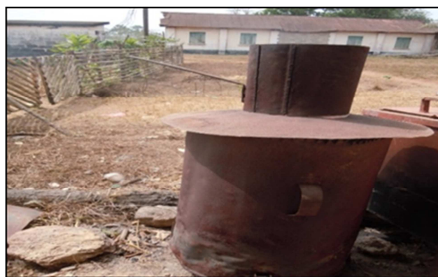
Figure 1. A digital photo of the locally-built Elsa Stove used to pyrolyze the Forest Lilac biomass used as biochar in the experiment.
