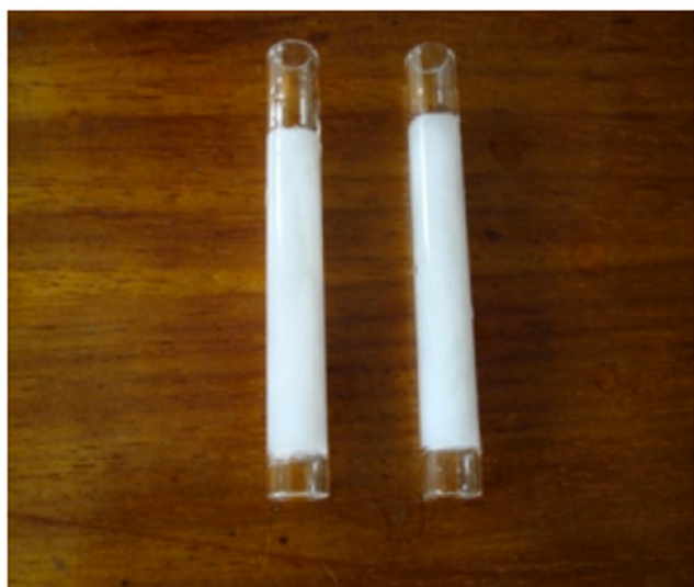
Figure 3. Cryogel in glass column after freezing, thawing and washing with water.
