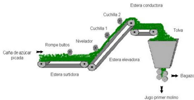
Figure 1. Transfer, preparation and feeding of the cane from the discharge to the entrance to the first mill.
