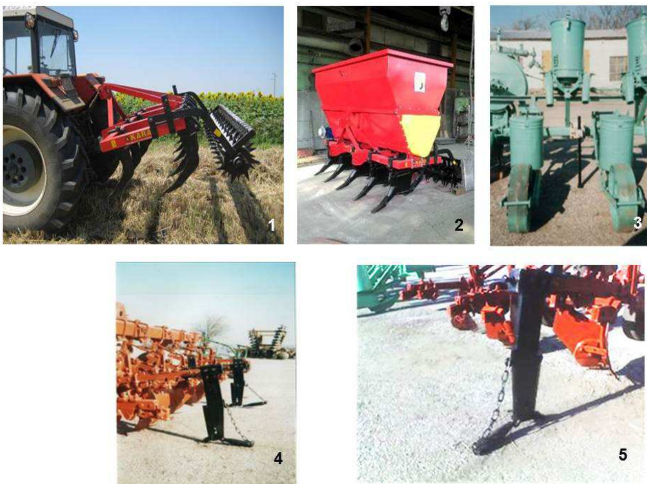
Figure 1. Machines and devices for the implementation of the advanced soil protection technology for minimum and unconventional soil tillage: 1- chisel cultivator CP-9; 2- specialized machine for vertical mulching; 3- sowing machine SPC 6 with slitting device; 4 - cultivator KRN 4.2 with cutting work bodies; 5 - A combination grooming device for implementation slits with ducts attached on cultivator KRN 4.2.
