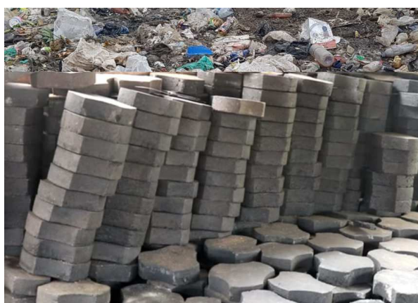
Figure 7. Paving stones made from plastic waste.
