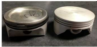
Figure 2. Low Compression vs. High Compression Pistons.
