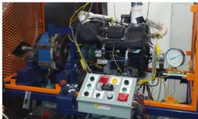
Figure 1. Kohler Command Pro ECH-749 and Test Stand
