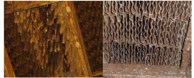
Figure 9. Corrosion of air preheater.
