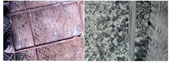
Figure 8. Fouling and plugging of air preheater.
