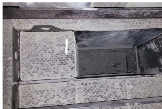
Figure 5. Fouling and plugging of catalyst.
