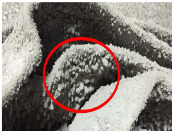
Figure 11. Dust Accumulates on Filters.
