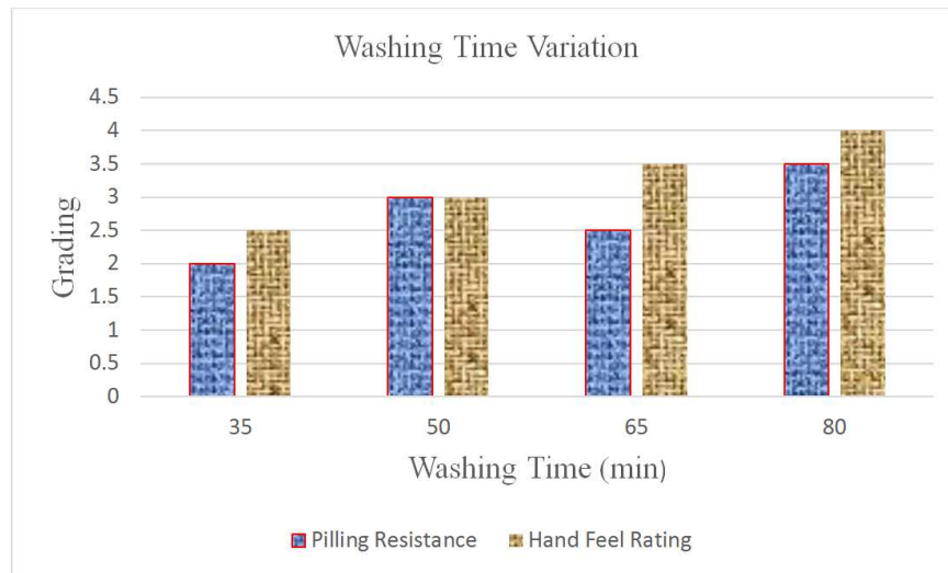
Figure 7. Variation of washing time on pilling resistance and hand feel rating of super white washed stretch denim fabric.
