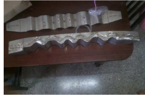
Fig 2. Sinusoidal test section.
