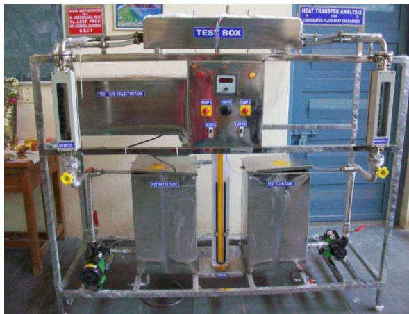
Fig 1. Plate heat exchanger setup.
