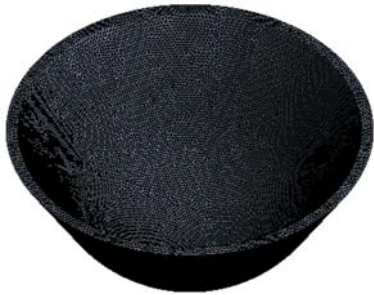
Figure 5. Mesh model of static region.
