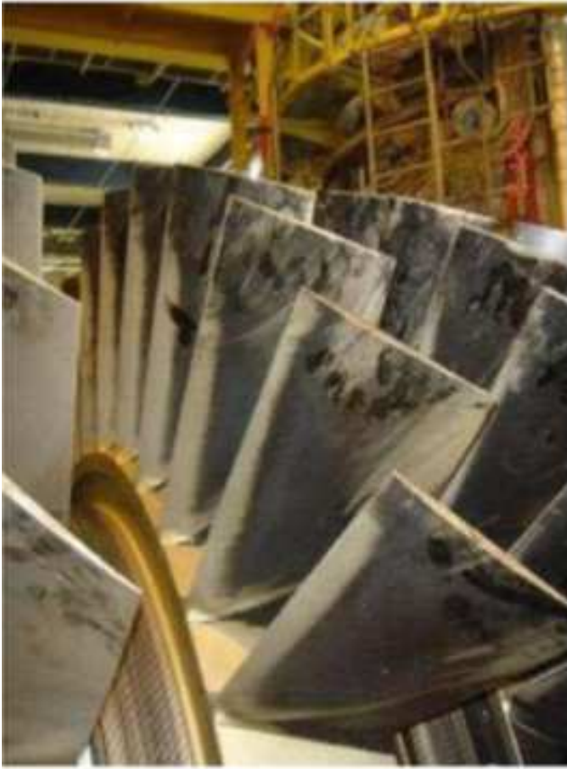
Figure 1. Example of fouling particles that attached on the airfoil of compressor blade [21].
