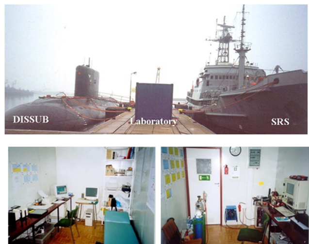
Figure 5. Above: arrangement of the main elements for the experiment; below: a containerized, portable laboratory.
