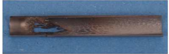
Figure 3-11. Erosion of the mixing tube wall
