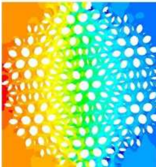
Figure 2.1-4. Pressure field in cross section of one idealized yarn.
