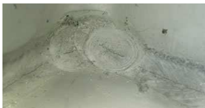
(c) crater cracks [3]
