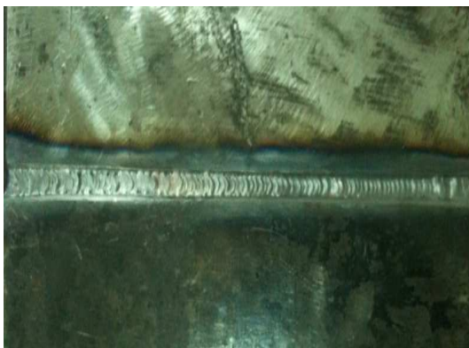
(b) Welding the back side by GTAW
