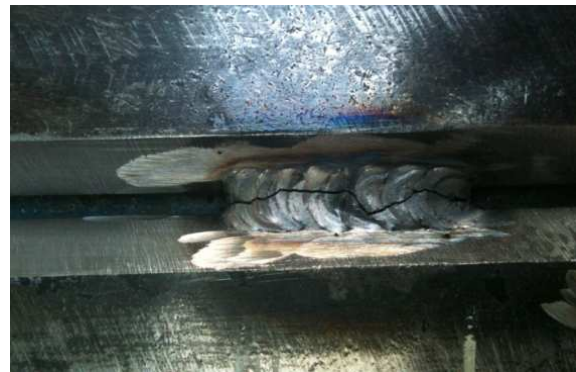
(b) Tackle the crack by GTAW process
