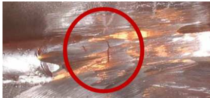
(b) Transverse cracks
