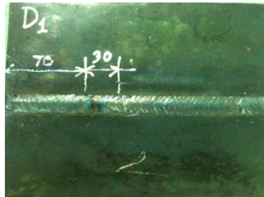
Figure 7. Cap layer welding.
