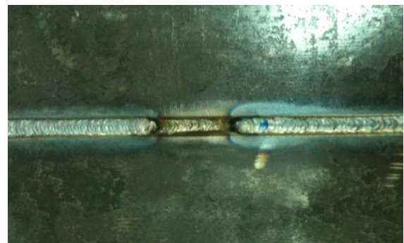
Figure 5. Welding at the other points in the fill pass
