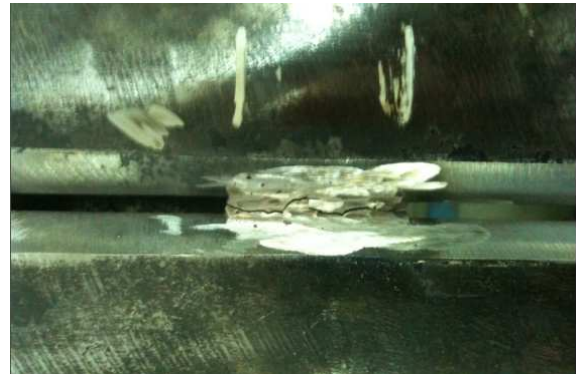
(a) Create the crack by SMAW process
