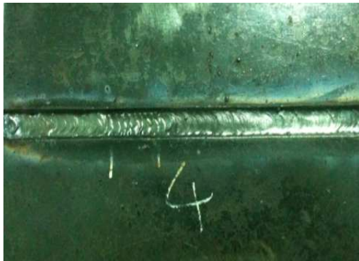
(a) Welding the front side by SMAW
