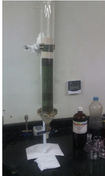
Fig. 2. Designed Green Sand Filter Unit.
