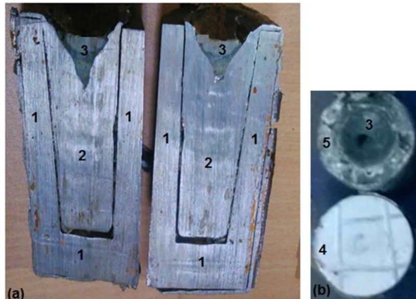
Figure 2. Design of large liquid steel sampler used in the present work.
