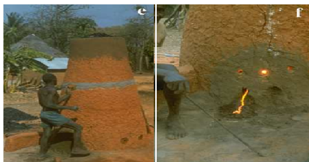
Figure 3. The Bandjeli furnace construction steps: (a) ground delimitation, (b) walls elevation at half height construction with the conical shape, (c) finished furnace with the tuyeres location holes and the gathered inputs charges around, (d) charges filling into the furnace and the set up of the tuyeres in the bottom, (e) external lining indication of the level of the ore within the furnace, 'the belly', (f) liquid slag flow 28 hours after the ignition of the furnace.
