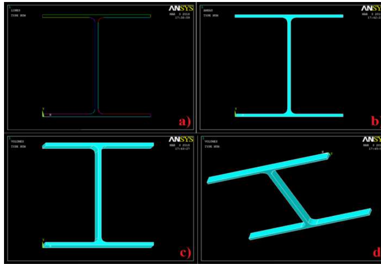
Figure 1. I-beam steel model's a) view of lines, b) creation of an area from lines, c) conversion to 3D, d) a different perspective of the 3D model.
