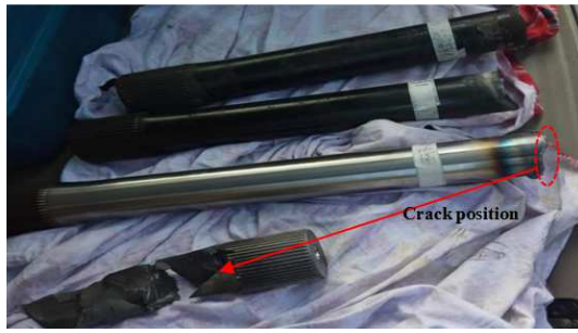
Figure 2. Crack position on torsion bar spline.
