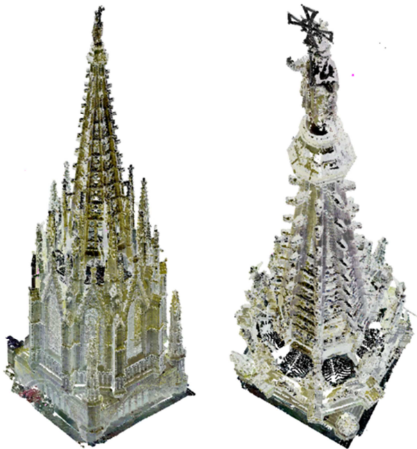
Figure 8. 3D laser scanning for the documentation of the spire (by TT12 Gabinet de Topografia i Construcció).
