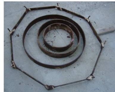
Figure 2. Corroded steel ties extracted from the spire.
