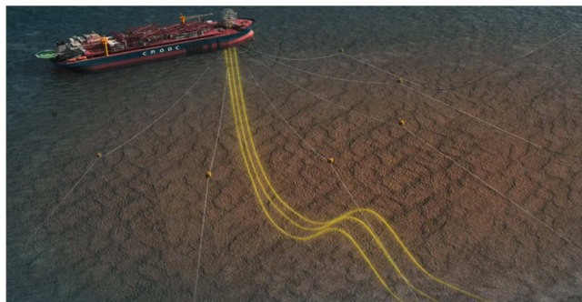
Figure 1. Structural form of anchor legs of FPSO.
