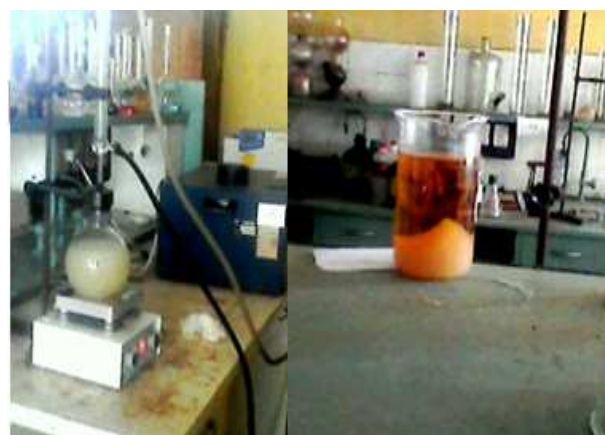
Figure 5. Transesterification reaction and biodiesel layer
