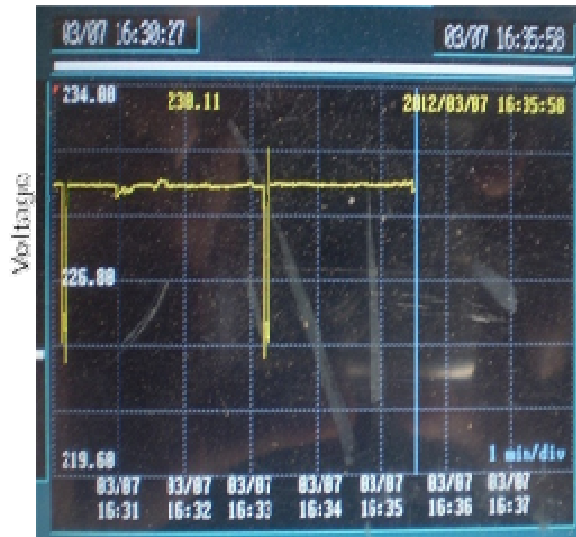
Figure 3: Time versus voltage curve with changing of load demand by voltage control scheme
