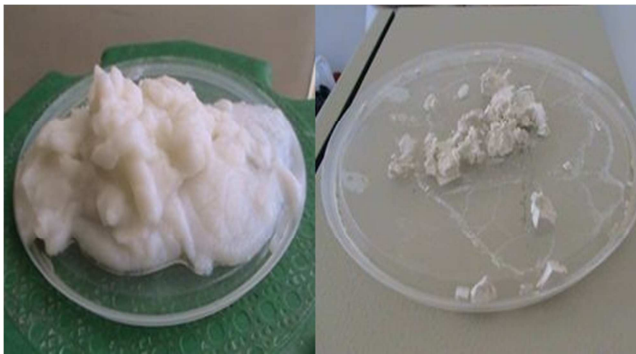
Figure 8. Sludge resulting from EC treatment using Aluminum electrodes.
