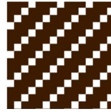
Figure 1. 3/1 twill fabric design RHT.
