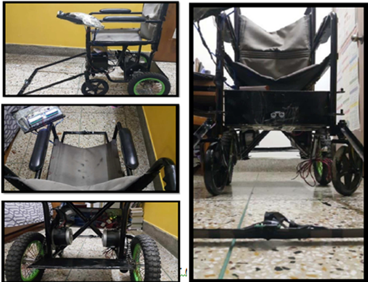
Figure 5. Intelligent Wheelchair (Side, Top, Back and Front view).
