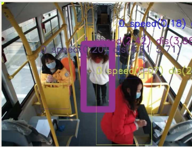
Figure 7. Implementation of the fast moving detection algorithm in bus.
