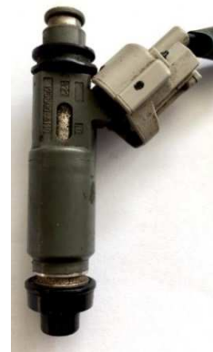
Figure 3. Fuel injector Denso 195500-3110.
