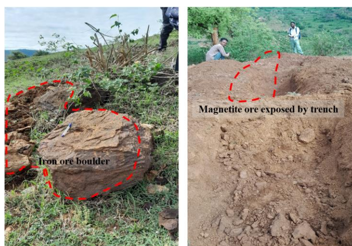
Figure 4. Variety form of iron ore body (exposed as boulders, gravels of iron fragmentation, vein type magnetite from the trench and surface floated) exposure of soka area.
