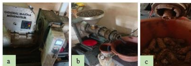
Figure 4. Worm screw press machine (a, b) and Jatropha cakes (c).
