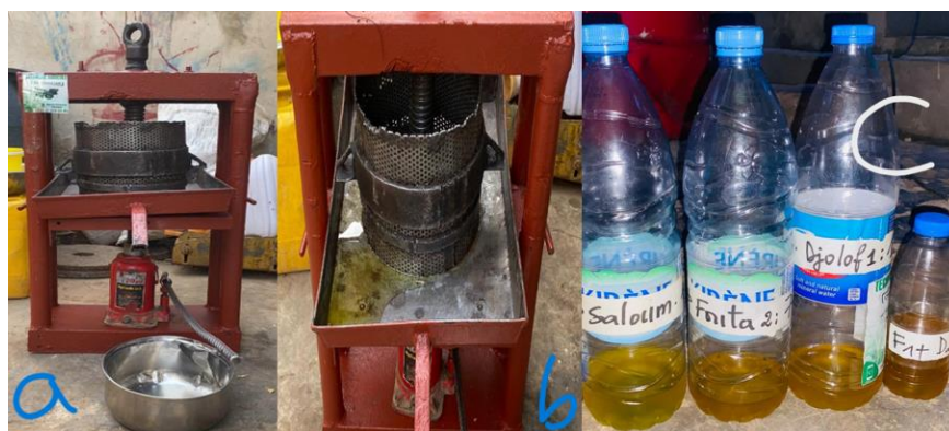
Figure 6. Hydraulic press (a = complete device; b = the oil outlet; c = extracted oils).
