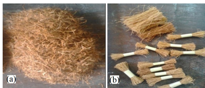
Figure 1. Short fibers ready for the production of the composite material. (a) Sisal short fiber mat. (b) NA Short fiber.
