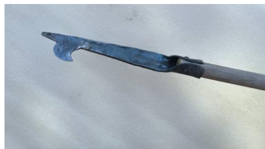
Figure 2. The Sonki innovated tapping tool which was developed by GRD, for tapping Acacia senegal . (Photo authorized Munner).
