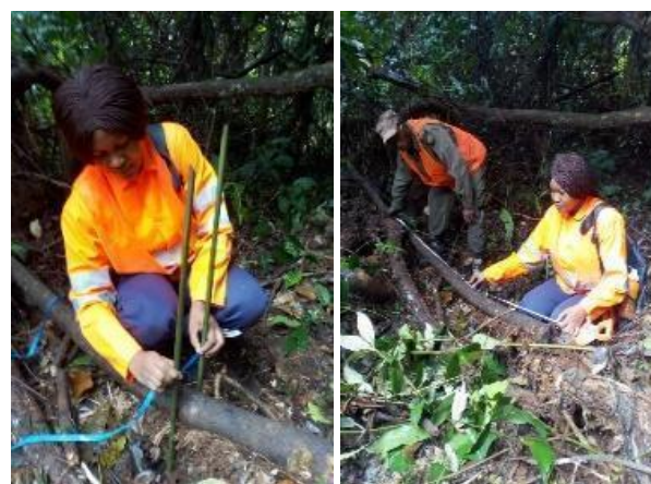
Figure 5. Measurements of dead wood lying on the ground (a. diameter and b. length).
