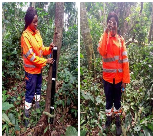
Figure 3. Measuring the height of standing dead wood with the relascope.
