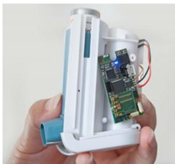
Figure 2. A Microcontroller in a Smart Inhaler.
