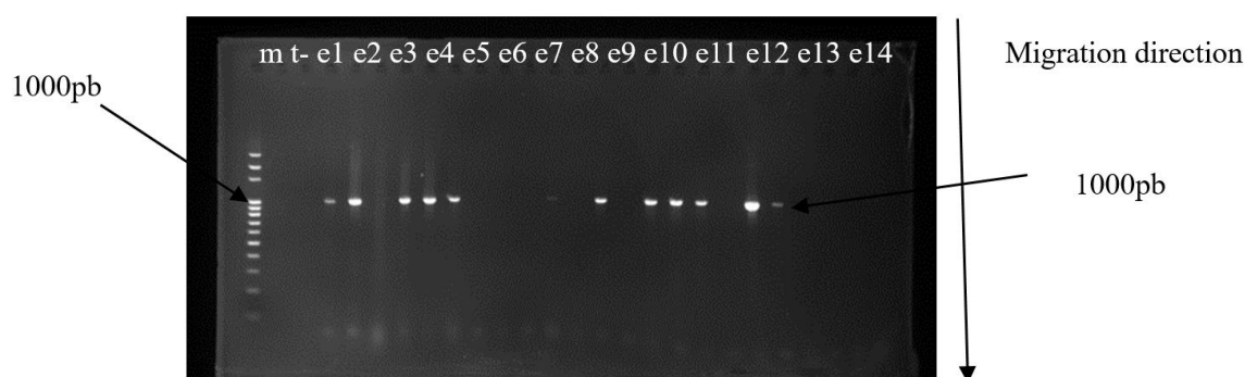
Figure 1. Electrophoretic profile of the amplicons of the bla CTX-M gene at 1000bp.
