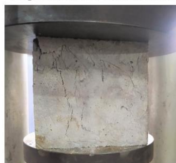
Step 4: Compressive strength test
