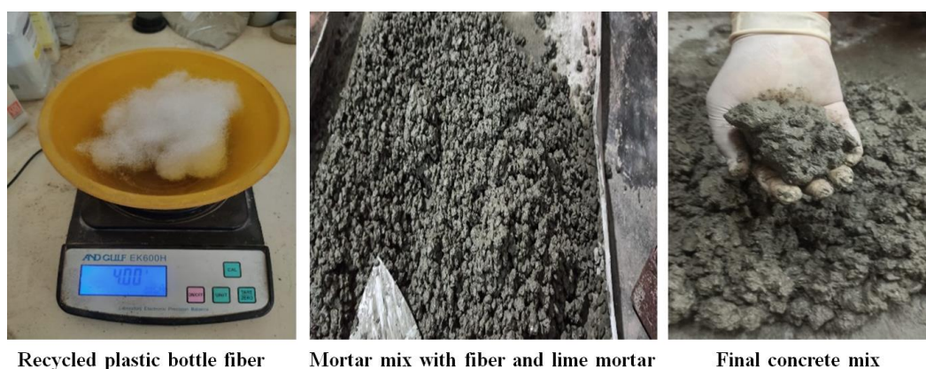
Figure 4. Concrete mix design with using of lime mortar and plastic bottle recycled fiber.
