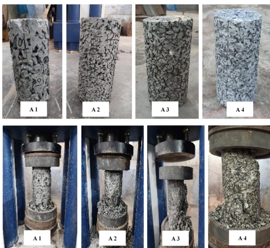
Figure 2. Compression testing of different specimen.
