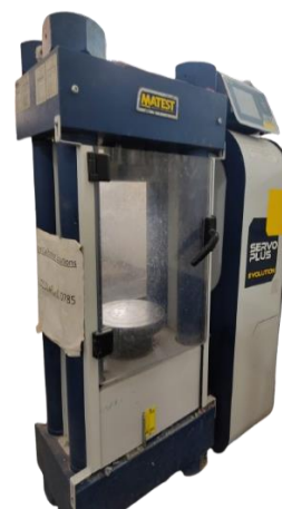
Figure 1. Matest Servo-Plus Evolution compression testing machine.
