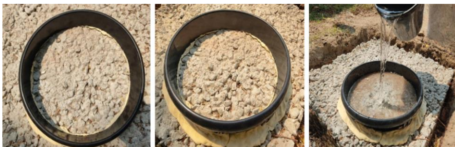
Figure 8. Infiltration test of Modified Pervious Concrete Pavement prototype.
