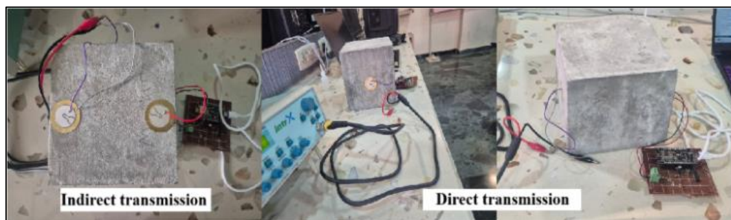
Figure 4. Experimental setup showing indirect and direct transmission configurations of PZT sensors.
