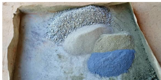
Figure 1. Coarse & Fine (Quarry Dust) Aggregates, Dust, Cement, and SF.
