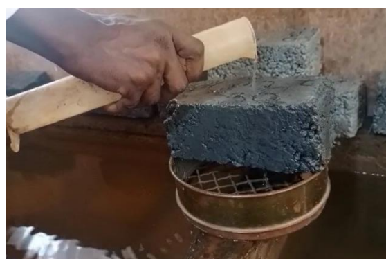
Figure 2. Permeability test on PPS.
