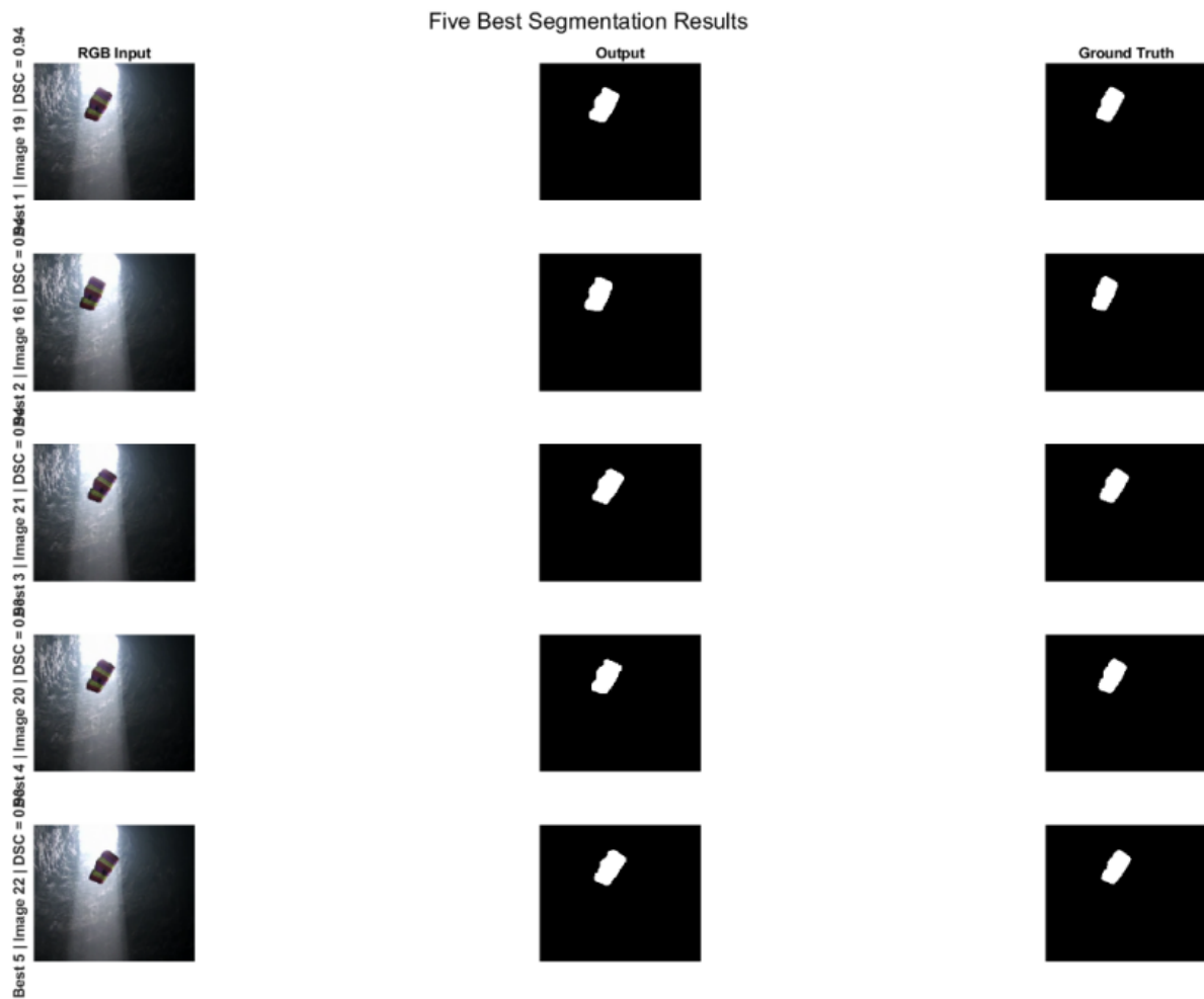
Figure 4. Five best segmentation results (DSC = 0.934–0.937). Each row shows the original RGB input (left), algorithm-predicted mask (centre), and ground truth mask (right). Well-lit, fully visible canopy with high chromatic saturation produces near-perfect boundary delineation.
