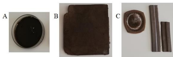
Figure 1. A: Sample of rubber produced from T. officinale , B: The state of the produced rubber after vulcanization C: Rubber samples after molding.
