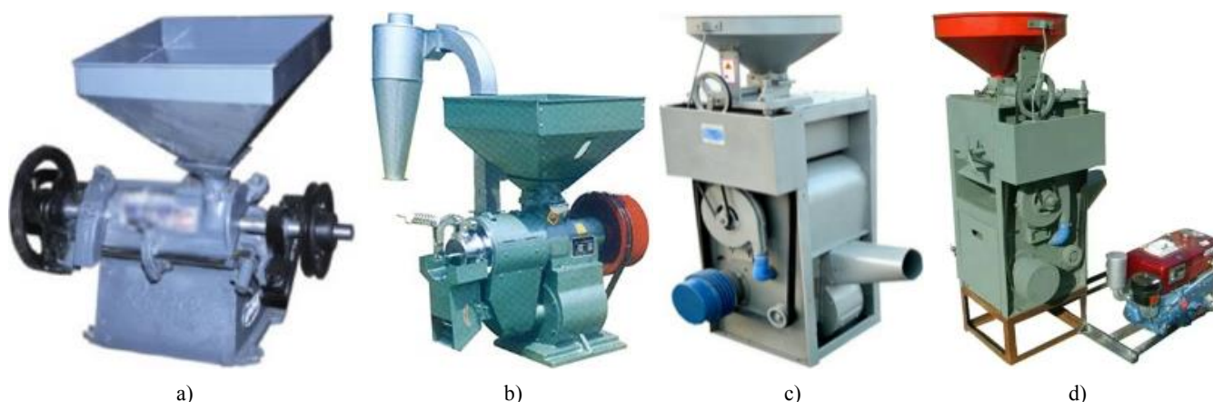
Figure 3. (a, b) Engelberg type rice mill, (c, d) SB type rubber roll rice mill.
