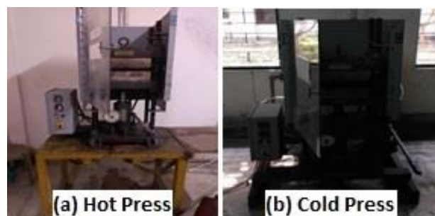
Figure 3. Carver Laboratory (USA) machine (a) Hot press (b) Cold press.
