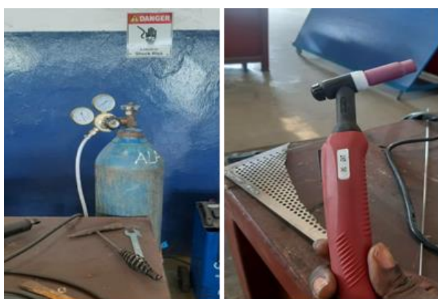
Figure 3. Tungsten Inert Gas Welding Equipment.
